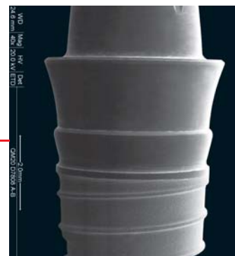
(Implant abutment interface showing no microgaps)
